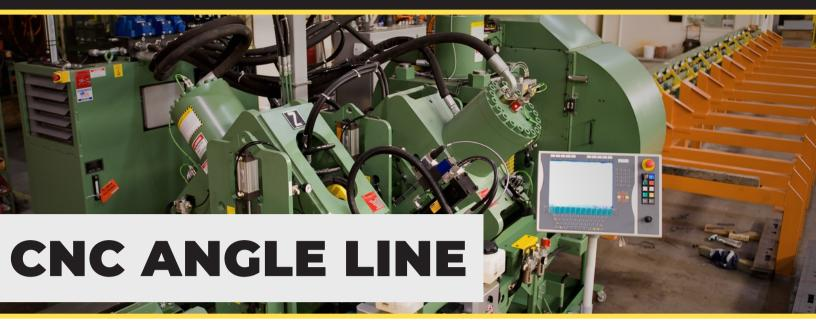
Clips, angles, gusset plates, and braces are essential components of the metal construction process. By utilizing our CNC angle lines, we improve structural steel fabrication efficiency by producing segments of angle and bar stock at a rapid speed and with no manual drilling.
